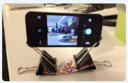
Fastening two binder clips to a strip of paper creates a simple and effective phone stand. Source: FixThePhoto
